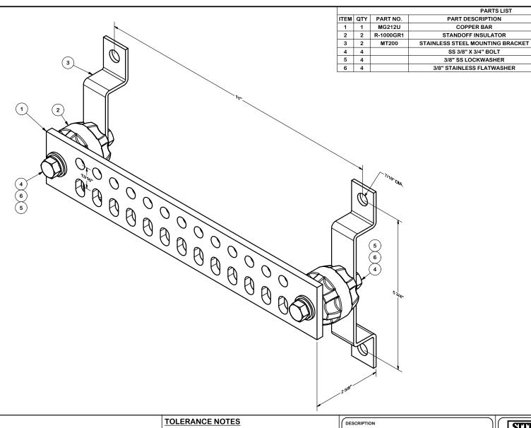
TOLERANCES ON DIMENSIONS, UNLESS OTHERWISE NOTED ARE: SAWED, SHEARED AND GAS CUT EDGES (\$ 0.030") ORILLED AND GAS CUT HOLES (\$ 0.030") - NO CONING OF HOLES LASER CUT EDGES AND HOLES (\$ 0.010") - NO CONING OF HOLES
